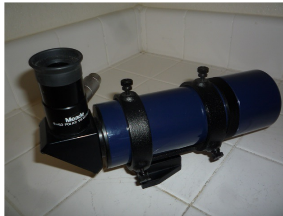
finder scope with illuminated reticle eyepiece
